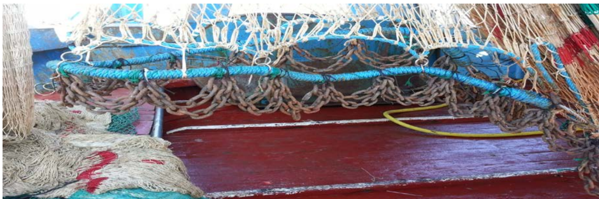
Figure XVI.1.3. In (a) Measurement of the distance between ballast chain bights (17 cm) and (b) of the inner height of the chain bightings (8 cm). Having such rigging the total weight of the chain must be around 120 kg. (c) supplementary chain (only one chain) of 15 kg (around 6.50 m and a diameter of 10 mm).
