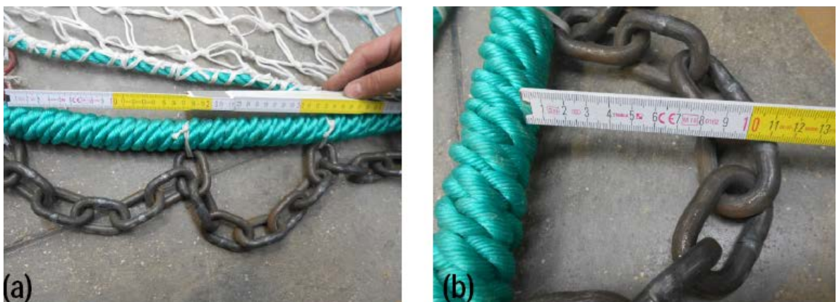
Figure XVI.1.2. In (a) measurement of the distance between the bolchline and the footrope (5 cm) and (b) between the bightings on the bolchline (50 cm).
