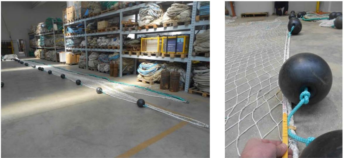
Figure XVI.1.6. Measurement of headline at wing tips. The measurement should start from the end of the wing to the end of the line. The headline in this part should be 6.00 m (d).
