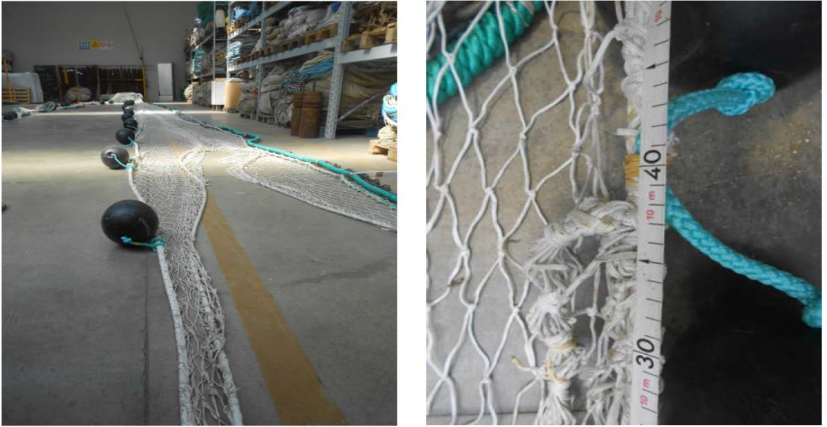
Figure XVI.1.5. Measurement of headline at wings. The measurement should start from the end of the bosom (see the transversal seams) to the end of the wing. The headline in this part should be 10.40 m (c).
